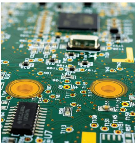
Brady Corporation's B-7634 masking film for PCB's offers excellent protection during electronic manufacturing processes, including wave soldering and hot air levelling. The polyimide masking film is ideal for auto-apply and can be removed cleanly.
