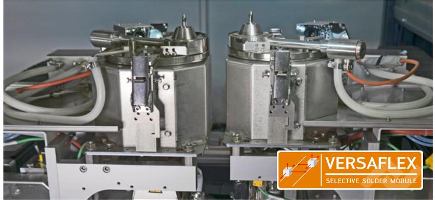
*VERSAFLEX module – 2 solder pots mounted on 2 independent axis systems*
