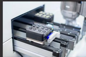
After depaneling and testing the PCB can be placed in different kind of storage or transport systems. Tray stacker, shuttle systems or WPC can be integrated to use the DIVISIO as island or as well in a line concept.
