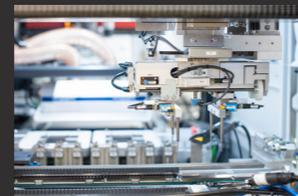
Product specific grippers allow the machine to handle all kind of PCBs. A Multigripper can handle up to 4 single PCBs at the same time to reduce the cycle time. Even rigid-flex PCBs can be handled.
