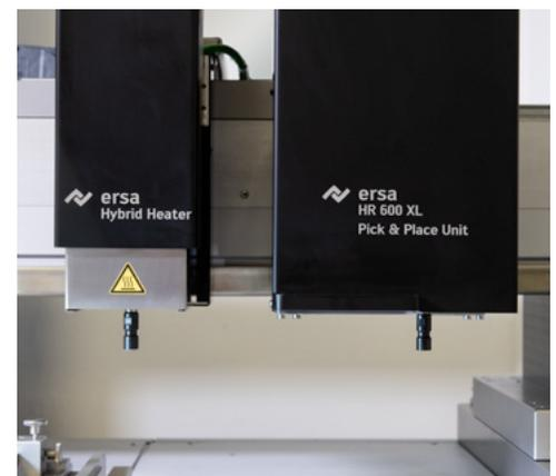
800 W Hybrid Heater right: Pick & Place unit, both with exchangeable nozzles
