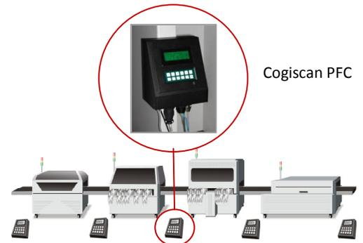
Since products are scanned at the entry of a process, the process validation, or error proofing, can be performed before the product is allowed to enter the process, without the need for any additional scanning steps.
